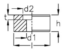
$$\begin{array}{lll} b & = 16 \\ d1 & = 7 \\ d2 & = 11 \\ H & = 10 \\ L & = 22 \\ screw = M6x16 \\ t & = 6.3 \end{array}$$
